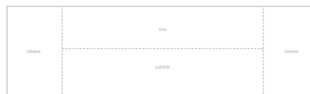
Figure 1. A summary tile presents a domain object with title, subtitle, and optional sidebars.
