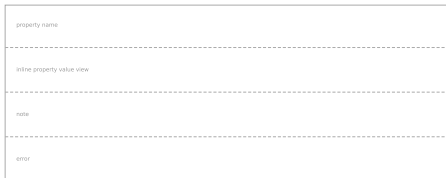
Figure 2. A property tile presents a single property as a key-value pair with optional note and error.
